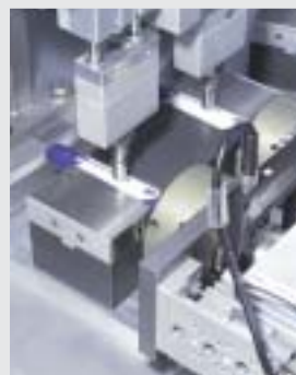
Testing station for penetration depth adjustment torque
